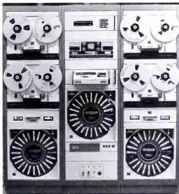
The SMC/Sono-Mag programming system, ESP-1, features 4000 events memory capacity; 20 stereo sources, with all source cards in place; and monitor and source cue included.
