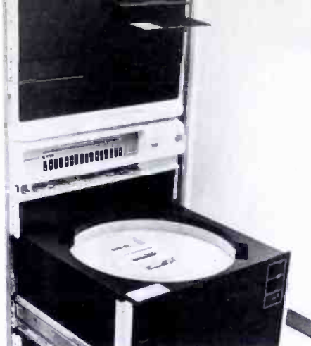
The Bloomington Broadcasting system uses both a floppy disc for electronic storage of historical material, and a hard disc for storage and fast, continuous access to current and future information.
